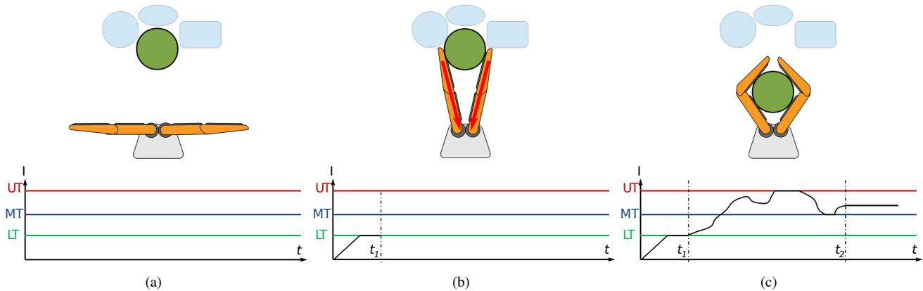
Fig. 3. *Grasp Execution Control*: As the open gripper closes in on the object (Left), the current through the opening motor is monitored. When contact is made (Middle), the actuated belts are switched on to pull in the object. The controller then strives to maintain the current in between two target thresholds by opening or closing the gripper during in-hand manipulation (Right).
