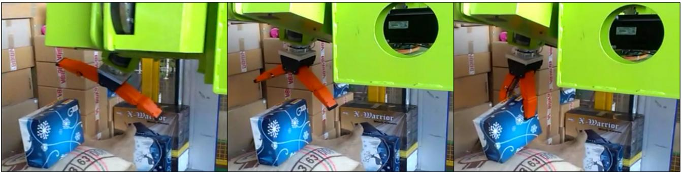
Fig. 4. *Grasp Execution*: The Velvet Fingers gripper on the Parcelrobot platform retrieves a box autonomously by employing the pull-in strategy.
