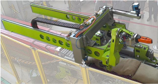
Fig. 1. *Parcelrobot and Velvet Fingers Gripper*: The Parcelrobot platform is located at the Bremer Institut für Produktion und Logistik GmbH (BIBA) in Bremen, Germany. Its kinematic structure comprises linear and rotary axes that cover a cylindrical workspace. Equipped with the Velvet Fingers Gripper it comprises an autonomous system for unloading shipment containers filled with randomly packed goods.
