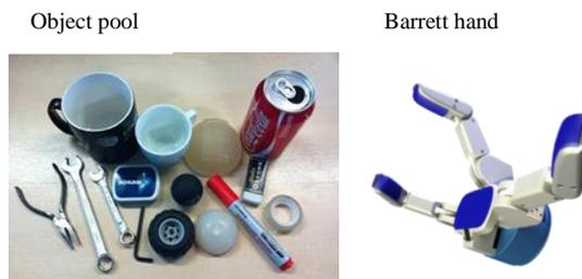
Figure 1. Depiction of the system to grasp objects. Left: object pool. Right: Barrett hand with tactile sensors.
