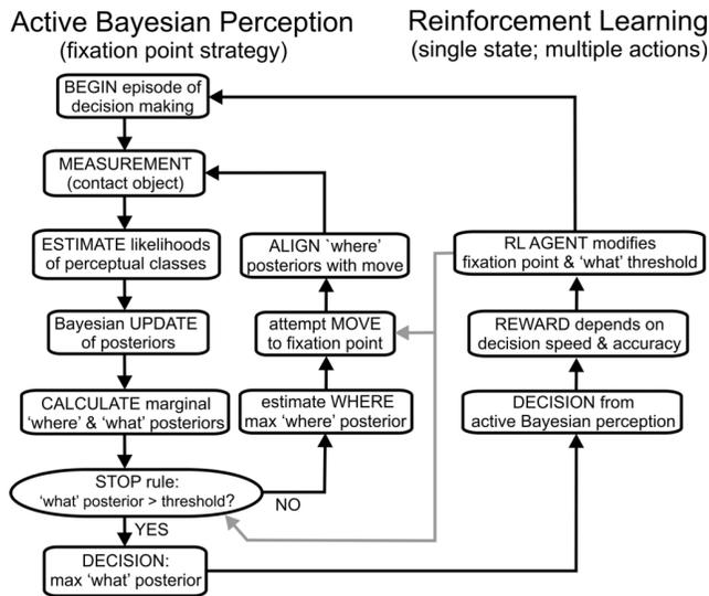
Fig. 2. Algorithm for active Bayesian perception with reinforcement learning. Active Bayesian perception (left) has a recursive Bayesian update to give the marginal ‘where’ and ‘what’ posteriors, allowing active control of the sensor position and decision termination at sufficient ‘what’ belief. Reinforcement learning (right) modifies the decision threshold and active control strategy based on reward information derived from the decisions.
