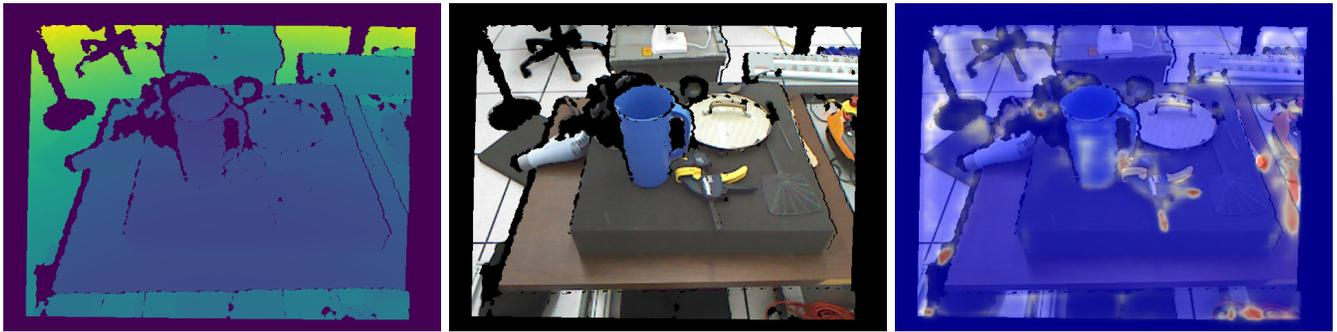
Fig. 2. Left: Depth image input to CNN, scaled to show in color. Middle: Color overlaid on point cloud depth image. Right: Probabilistic map output by CNN, highlighting regions that resemble handles for grasping.
