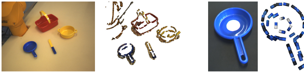
Figure 3.2: Sparse-stereo reconstructions of object edges [Krüger et al., 2004, Pugeault, 2008]. Each cylinder corresponds to an edge-segment descriptor. The axis of a cylinder is aligned with the direction of the modeled edge. Each cylinder bears the two colors found on both sides of the edge in 2D images. For clarity, the reconstruction of the toy pan (right side of the figure) only shows a fraction of the descriptors available for this object.
