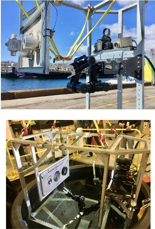
Fig. 3. Perception head, test panel, and robot manipulator mounted on a rigid frame in the relative configuration used for the experiment of Fig. 6.
