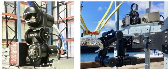
Fig. 1. Sensor head and articulated robot. Left: sensor head combining two cameras, an LED light (red-colored housing) and a sonar (above the light and cameras). Right: Cameras, pattern projector (grey metal housing), robot arm.
