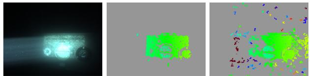
Fig. 8. Camera image (left) and disparity (middle and right) captured at  $t = 2.5$  hours (medium turbidity), with a 0.16s shutter speed and 24px block pattern. The middle image illustrates a disparity map computed with standard block matching, while the rightmost image was computed with SGBM. Green pixels are approximately 1.1m far from the cameras. Red pixels are less than a meter from the cameras; blue pixels are further than 1.2m.
