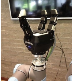
Fig. 3. Robotiq three-finger gripper equipped with tactile sensors. The proximal sensors are currently not functional.
