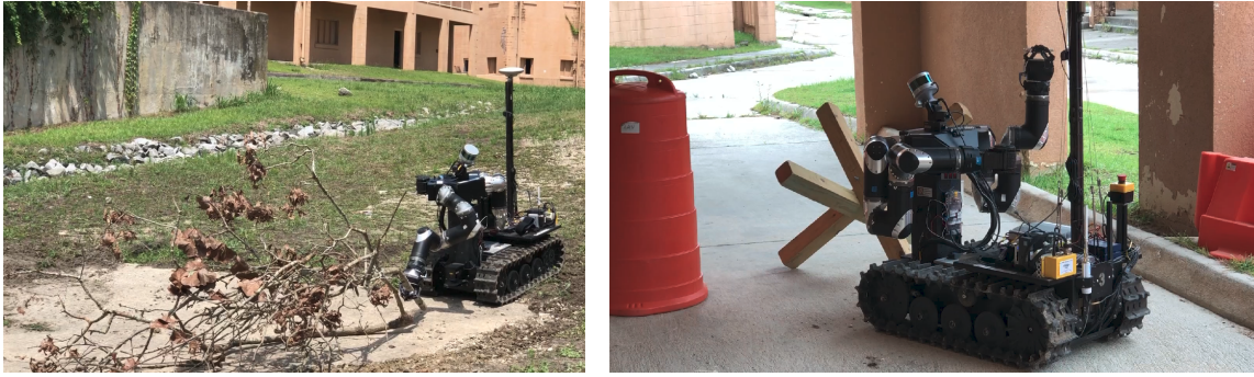
Figure 9. Left: RoMan dragging a tree branch. Right: RoMan in front of a Czech Hedgehog.
