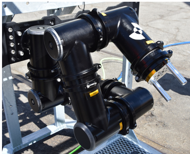
Fig. 3. The assembled limb in the Pre-manipulation-1 pose mounted to a test frame.
