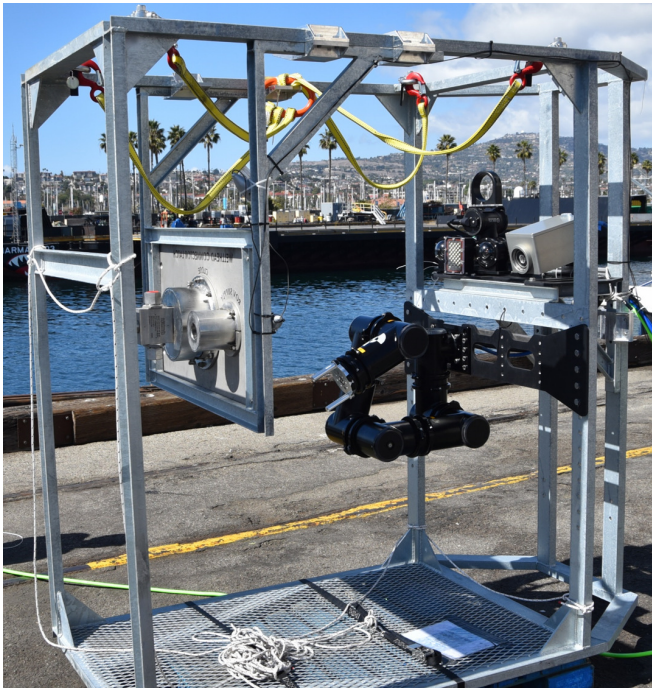
Fig. 5. The AquaSimian Limb mounted to a test frame with a subsea task panel for field testing.
