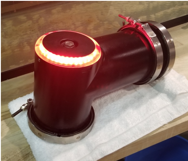
Fig. 8. The Light Lid warning of a detected leak through visual display of a red indicator light.
