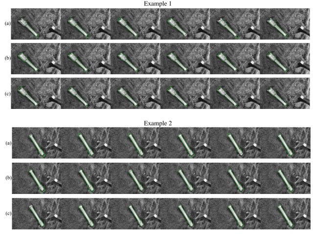
**Figure 7**. Visualized pose estimates for a subset of all trials using 10k samples for two arbitrarily chosen test examples: (a) Uniform sampling, (b) geometry-constrained sampling (without learning), and (c) geometry-constrained sampling followed by learned sampling. The rendered boundaries are highlighted in green-and-black double lines on the gray-scale images. (Best Viewed in Color)
