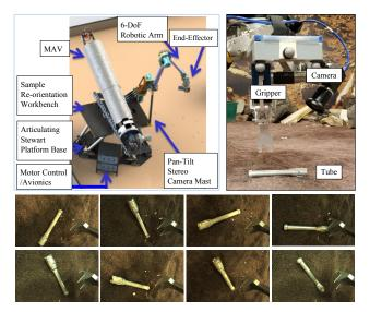
Figure 1. (Top-left) The MSTT platform, (Top-right) the toolcam at the end-effector, and (Bottom Rows) examples of tube images taken from the camera.
