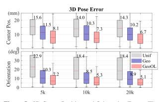
**Figure 5**. 3D Center Position and Orientation Errors: The numbers indicate the median values. (Note for boxplot: The red center line indicates the median, the box indicates 25 to 75%, and the whiskers indicate 1 to 99% of the data.)
