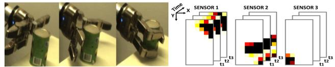
Fig. 1. (Left) Example of grasp execution with the three finger Schunk Dexterous Hand (SDH) [3]. (Right) Tactile measurements create a sequence over time in which information in consecutive frames is correlated.
