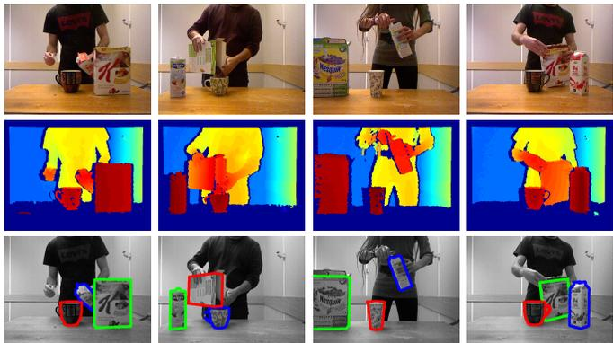
Fig. 3. Examples taken from the dataset. The first two rows show the raw RGB-D data while the last row shows the results of the tracker used. For more examples please refer to the supplemental material.
