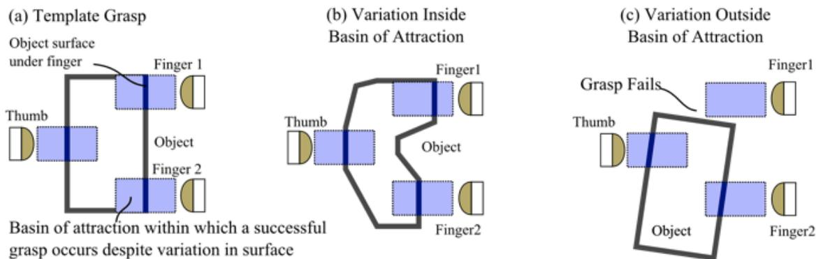
Figure 3: Analysis of all sources of variation generates a “basin of attraction” for variation from the original template grasp. If object surfaces fall within this range under the current variations in geometry, pose, arm inaccuracies, etc., the grasp will succeed.
