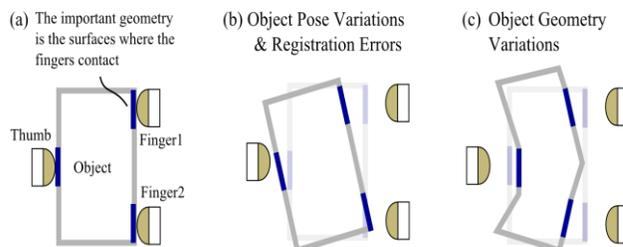
Figure 2: Variations in object geometry from object pose, geometry, registration errors, and perceptual uncertainty
