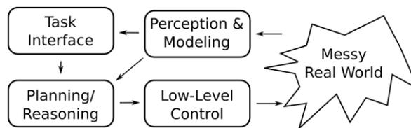
Figure 1: System breakdown of a typical grasping robot.
