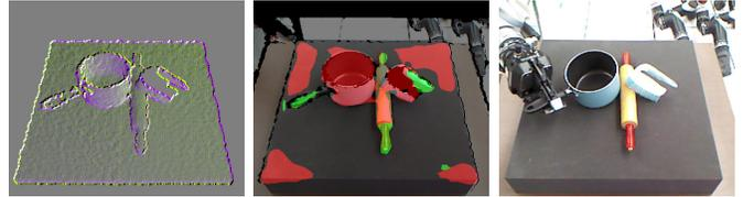
Fig. 1. Grasping for a *transport* task. Left: Depth gradient, input to the CNN. Middle: the green overlay indicates task-compatible regions encoded by the CNN (here: grasp handles only). Right: Planning and executing a 7DOF grasp (pose and preshape) within a compatible region.
