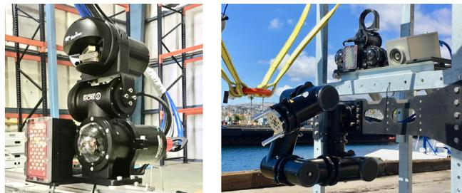
Fig. 1. Sensor head and articulated robot. Left: sensor head combining two cameras, an LED light (red-colored housing) and a sonar (above the light and cameras). Right: Cameras, pattern projector (grey metal housing), robot arm.
