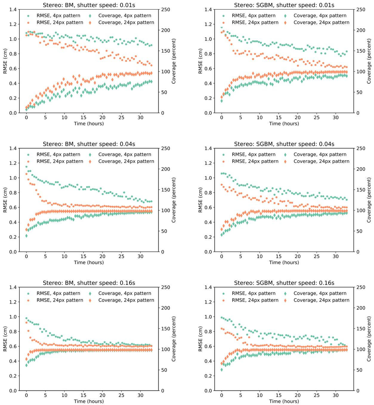
Fig. 6. Accuracy (RMSE) and coverage of stereo reconstructions with different shutter speeds and projected patterns. The plots show a systematically-sampled subset of the data for clarity. Refer to Fig. 4 to relate time to turbidity.
