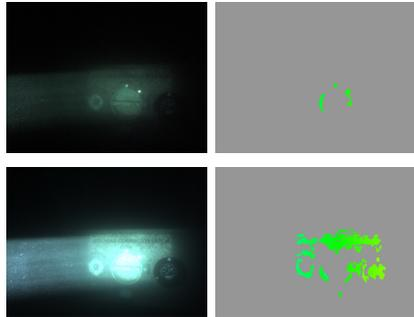
Fig. 7. Camera image (left) and disparity (right) captured at  $t = 8$  minutes (high turbidity), with shutter speeds of 0.01s (top) and 0.16s (bottom). Both top and bottom images were captured while projecting the pattern with the largest block size (24px).
