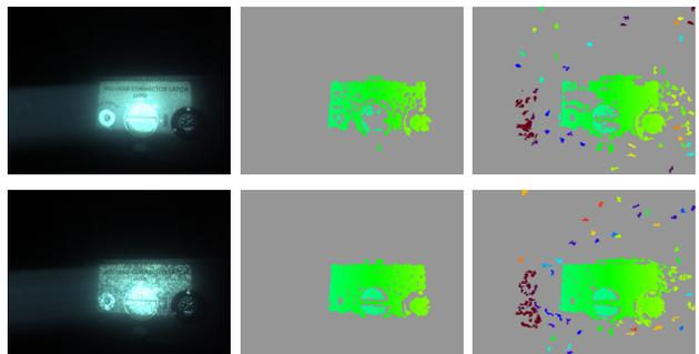
Fig. 9. Camera image (left) and disparity (middle and right) captured at  $t = 33$  hours (low turbidity), with a 0.04s shutter speed, and 4px and 24px block pattern for the top and bottom row respectively. In each row, the middle image illustrates a disparity map computed with standard block matching, while the rightmost image was computed with SGBM. Green pixels are approximately 1.1m far from the cameras. Red pixels are less than a meter from the cameras; blue pixels are further than 1.2m.
