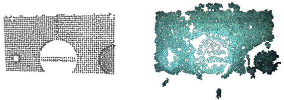
Fig. 5. Ground truth structure (left) and stereo point cloud (right). Ground truth was established via manual measurements. The ground truth panel only contains points that are within the projection cone of the pattern projector, and within the frontal plane of the panel.
