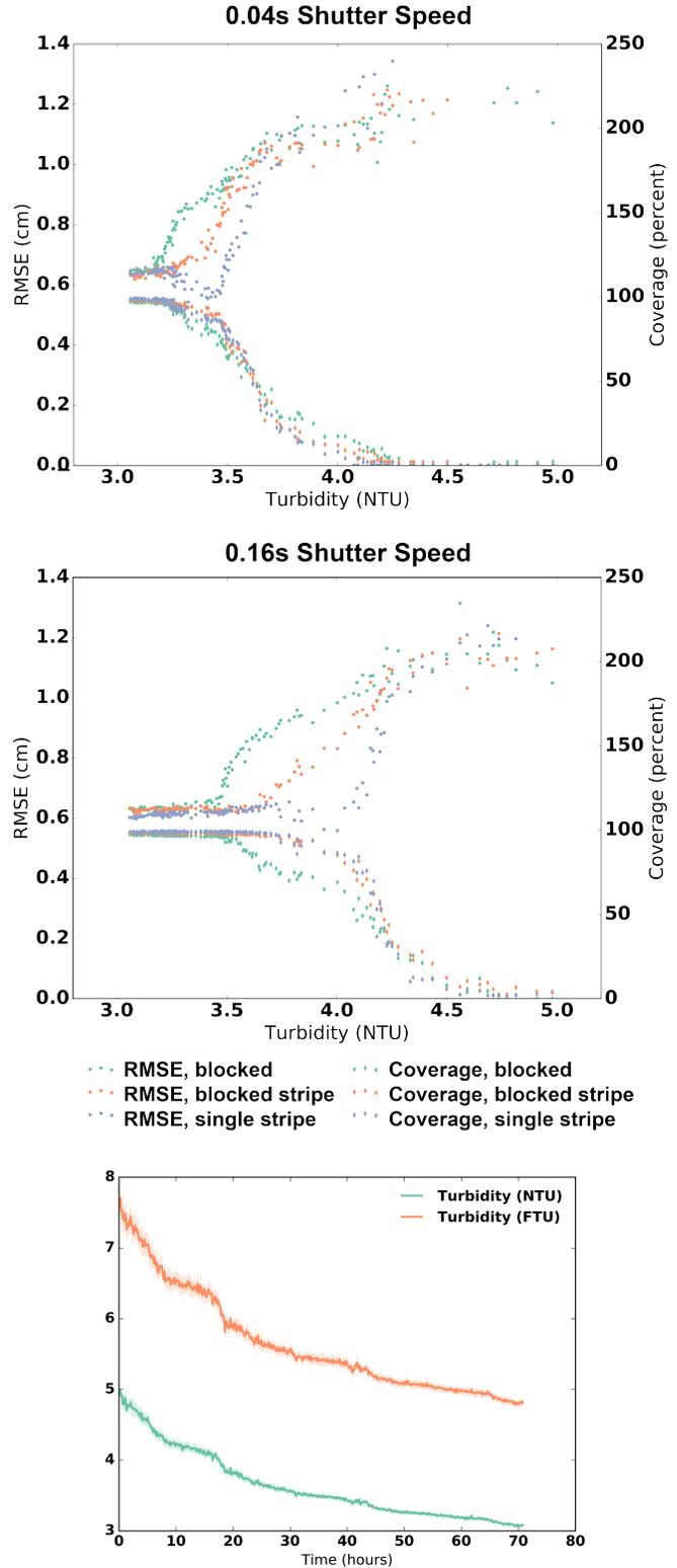
Fig. 5. Plots from the underwater test. The top two images show RMS and Coverage as a function of turbidity for shutter speeds of 0.04 and 0.16 seconds. The bottom image shows the turbidity measurements throughout the 70 hours of testing.
